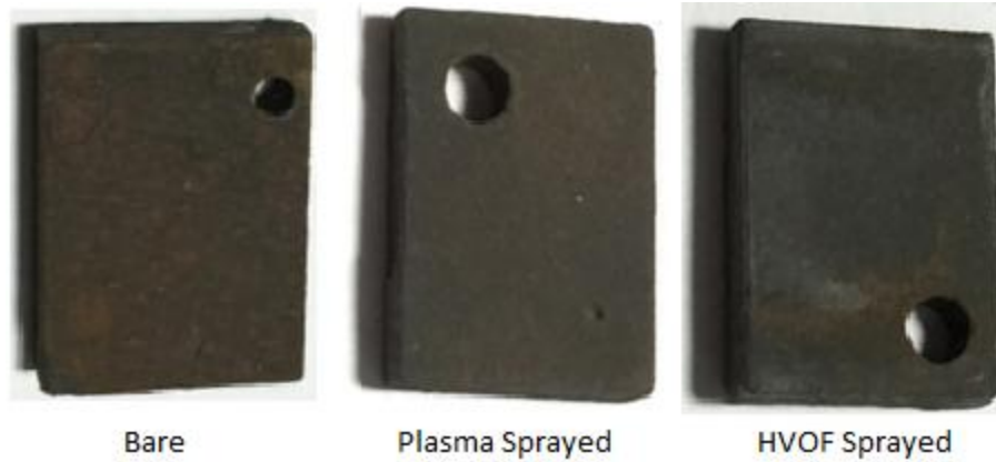
Fig.7. Macrographs of the bare, Plasma and HVOF sprayed specimens subjected to actual boiler environment.
